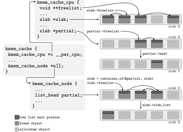
Figure 1: `kmem_cache` layout for the SLUB implementation.
