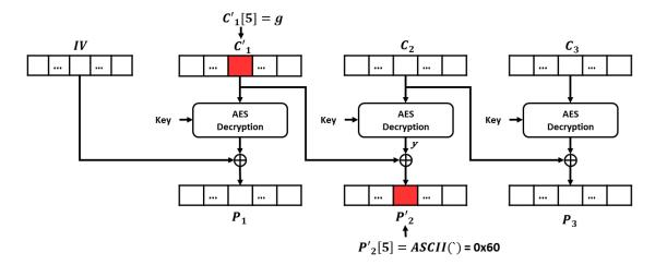
Figure 4: Syntax-oracle attack to extract the plaintext,  $P_2[5]$ . Before the attack,  $P_2[5] = C_1[5] \oplus y[5]$ . When  $C_1'[5] = g$ , suppose **SO** returns 1, i.e.,  $P_2'[5] = 0x60$ . Since,  $P_2'[5] = C_1'[5] \oplus y[5]$ , so  $P_2[5] = C_1[5] \oplus 0x60 \oplus g$ . ( $P_2'$  and  $C_1'$  represent the modified plaintext and ciphertext block.)
