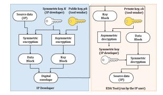
Figure 3: Work flow of the P1735 standard.
