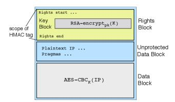
**Figure 1:** A P1735 ver. 2 *Digital Envelope.* The Rights Block contains the RSA-encryption of an AES key, which is used to encrypt the sensitive portions of the IP with AES-CBC mode. Note that only the Rights Block is covered by the authentication mechanism.
