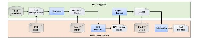
Figure 2: System-on-chip (SoC) design flow.
