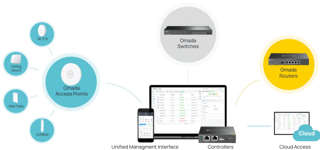
Figure 2 – Omada devices using a local, on-premises controller (source: tp-link.com)
